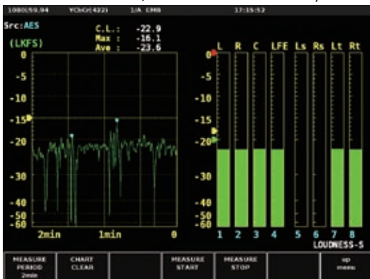
Loudness display (with the LV 5770SER41 installed)
