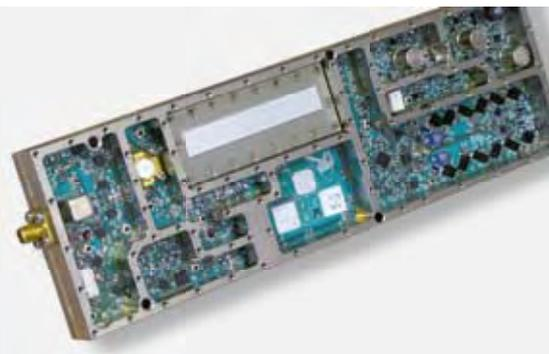
figure 3: RF section of the IZT S1000
