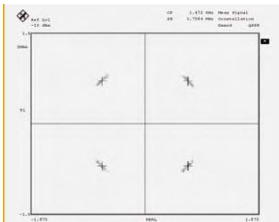
**figure 9:** QPSK constellation affected by phase noise
