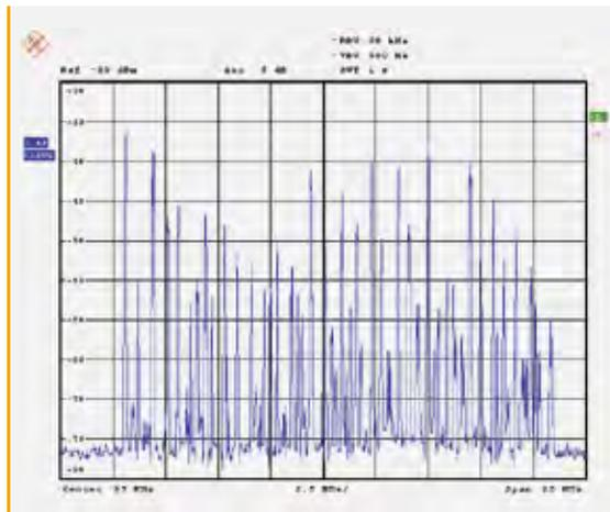
figure 5: Recorded FM broadcast spectrum
