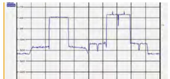
figure 13: Full Sirius XM Radio signal using eight virtual signal generators
