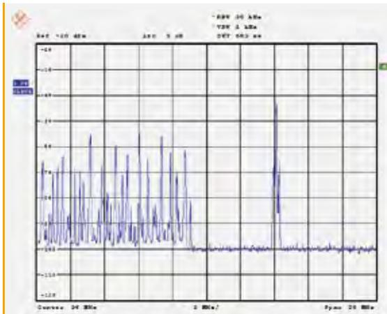
figure 10: Recorded FM broadcast spectrum combined with one HD Radio signal
