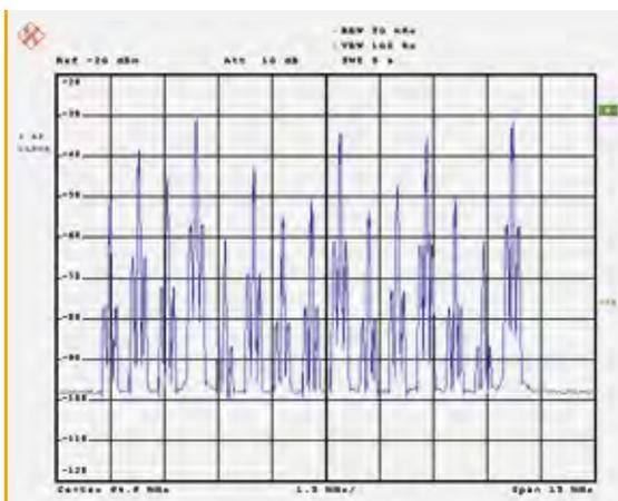
figure 12: Fifteen HD Radio signals
